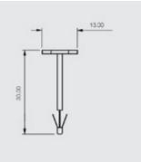
Renderplas plastic fixing pins for insulation board offer a fast simple way to install mesh beads on insulation panels. The carefully engineered tree design provides maximum grip and an exceptionally small piercing point making them very easy to use
